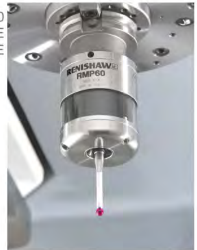
RENISHAW RMP-60 AUTOMATIC WORKPIECE CENTER MEASURING DEVICE
