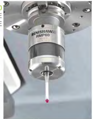
RENISHAW RMP-60 AUTOMATIC WORKPIECE CENTER MEASURING DEVICE
